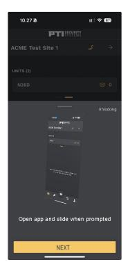
Unlocking PROEdge (When prompted by the app, slide the button on the app to open the lock)
